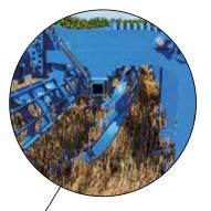
**Levelling harrow** to ensure optimal levelling
