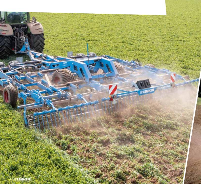
Right after the harvest is the time for preparing a basis from which the next crop can develop optimally. The Koralin 9 cuts stubble both vertically and horizontally across the full working width to promote rapid microbiological decomposition. At the same time, it incorporates harvest residue at a very shallow depth. This encourages the even emergence of weed seeds and volunteer cereals while also reducing evaporation. As a result, water in the soil is retained for catch crops.
